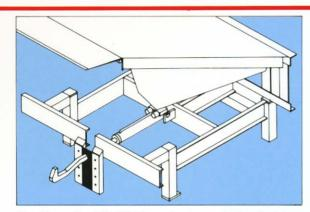
The PowerHook<sup>TM</sup> KS7 is a stand-mounted restraint that's ideal for retrofit or new construction. Front legs of stand are recessed so that concrete or block wall can be constructed to give your dock a clean, finished look.
