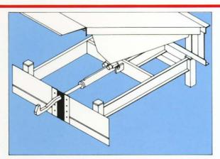
The PowerHook™ KS6 is mounted on a stand that slides into any new or existing full-depth pit. It's easy to install. . .just weld it into position and run power to it.
