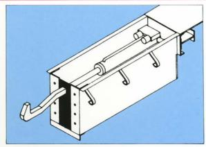
The PowerHook™ KS5 pan-type truck restraint is an economical retrofit for hydraulic dock levelers. All that's required is a minimum 44" dock height.
